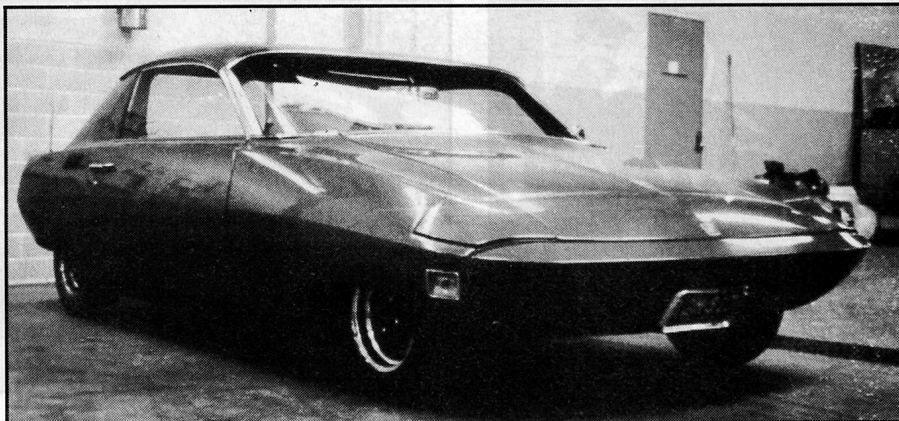
The famous commuter car that Adams developed into a fully functional prototype. It was a three-seater, and was powered by the X4-2 cycle engine.
