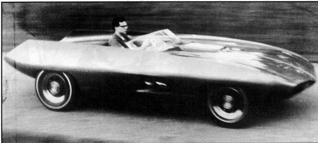
This beautiful two-seat sports car, called the ViVante, was designed by Adams, and he had it built for himself. It used a 370-cubic-inch Pontiac engine and four-speed transmission, along with Pontiac eight-lug wheels and a hand-formed aluminum body.
