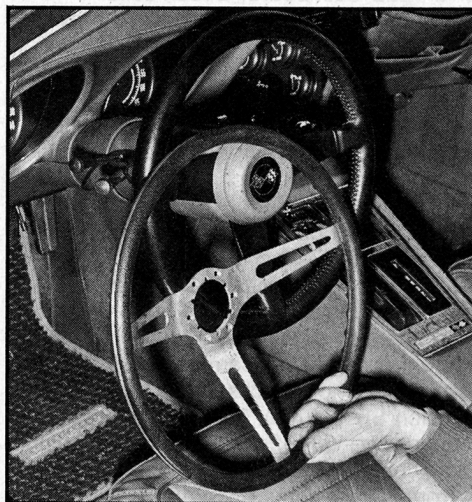
Adams replaced stock steering wheel with 14½-inch-diameter, leather-wrapped VSE steering wheel. Reducing wheel diameter increases effort slightly.
