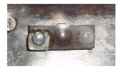
3. After removing the glass, clean off the silicone residue from the back of the glass and from the 4 mounting pods on the housing. Also, clean off the plate and rivets that hold the mirror post ball in place. This area needs to be completely clean.
